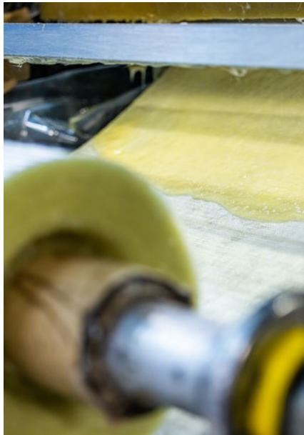
The impregnation unit evenly saturates the GRP fabric with reactive resin
